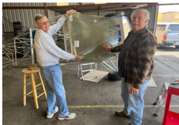
Lee reports that the Bearhawk windscreen which they are in the process of fitting comes out very nicely from the factory. It's almost a perfect fit right out of the box. Lee's helper Bill Lawrence is assisting on the filling of the screen. More to report later.
