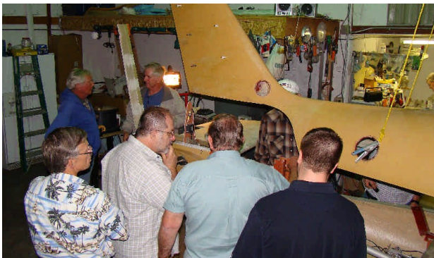
Carl Johnston's Europa below with construction help from Rick Lambert. The top shell of the fuselage has yet to be attached to the bottom:
